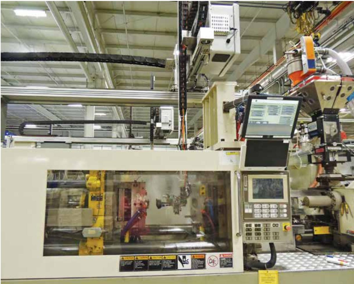
arm tooling (EOAT) extracts the plastic parts from the molds. The EOAT is equipped with vacuum cups that remove the finished parts and drop them on a conveyor. Average cycle times for this process range anywhere from 10 to 30 seconds, depending on the application.
