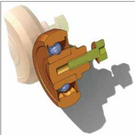
**Rollon's Compact Rail ball bearings are permanently lubricated and sealed within the rollers, which isolates these small rolling elements from contaminants.**
