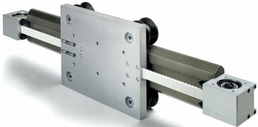
tion or maintenance. The large sized rollers and the convex profiles make it the ideal solution for applications in the harshest environments, such as ceramic processing or welding. The plastic compound coating of the rollers also allows the smaller debris to be absorbed without adversely affecting its sliding quality.
