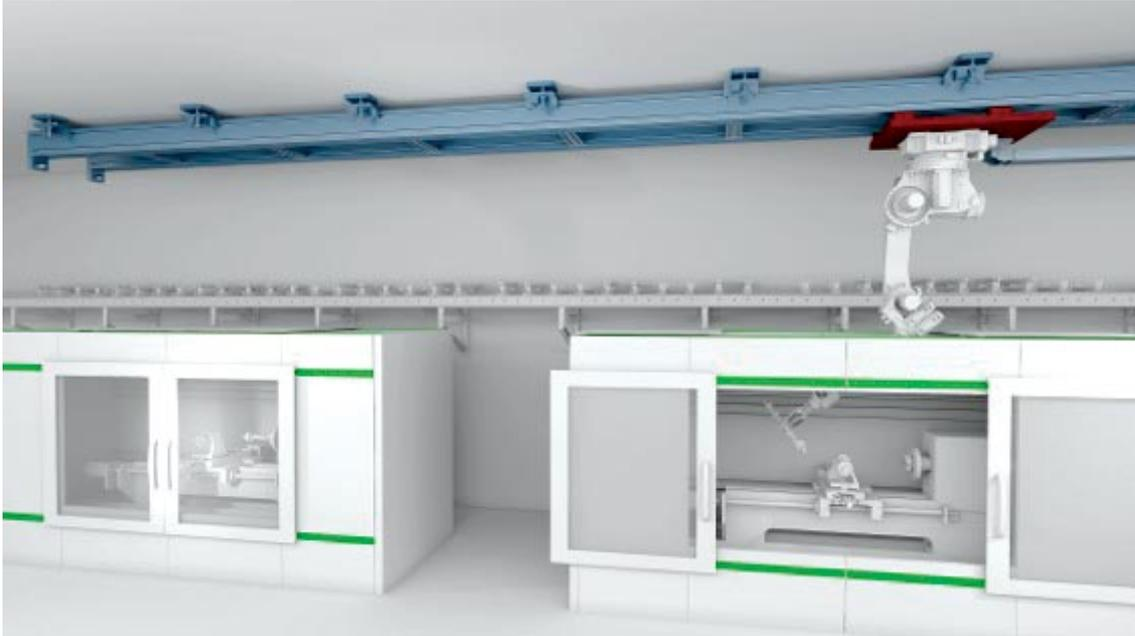
This is a solution that is capable of transporting large robots with potentially infinite strokes
