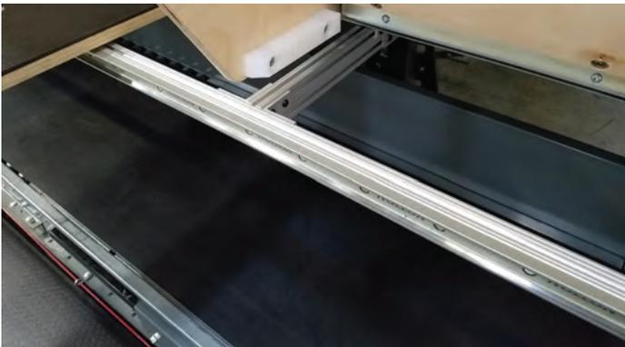
*The linear bearings used in the packaging module had to handle very high loads. A 150-pound package placed at the end of a table, for example, would create a 600-pound moment load on the supporting structure.*
