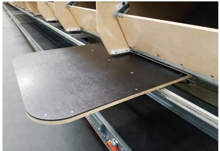
*The packaging module includes tables, which are made of strong ply and are capped with an ABS plastic. The tables were mounted onto a Rollon linear guide, which was inserted into a standard aluminum extrusion.*
