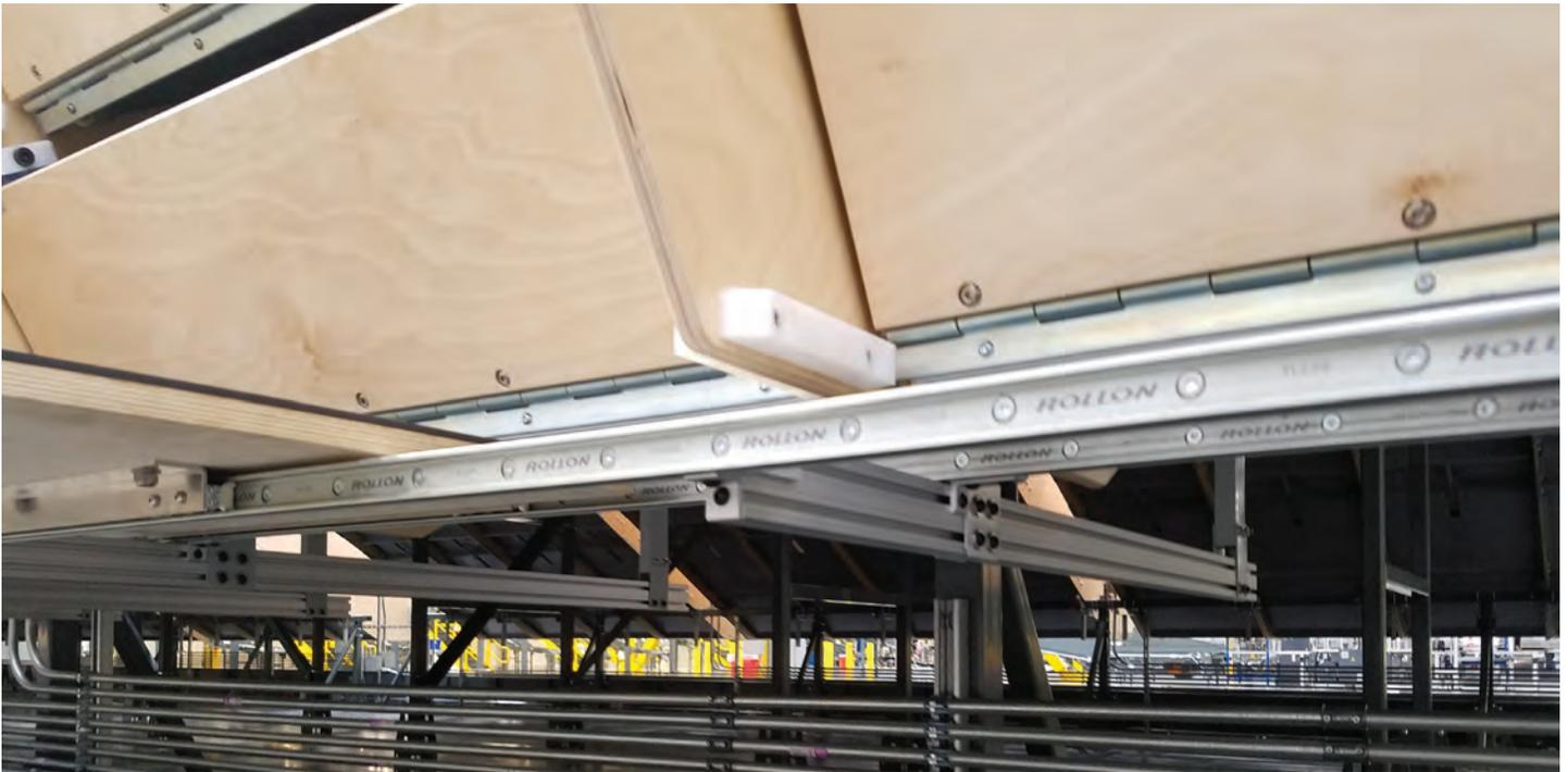
*Though limited by challenging design constraints, N-III created a supporting structure that mounts underneath a distribution center packaging module, integrating an arrangement of plywood, aluminum extrusions and Rollon linear bearings.*
