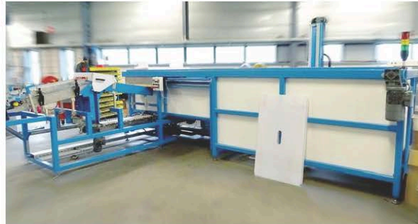
Following Rollon's suggestions, the Corenso machine is made with Compact Rail linear rails.
